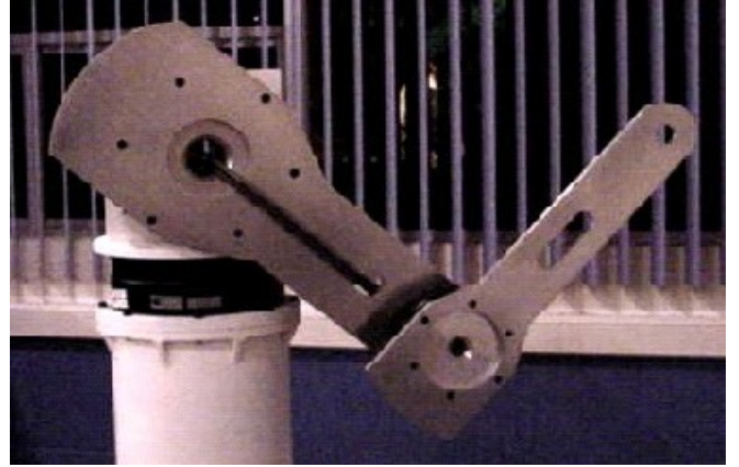
Figure 2: Robot Manipulator of 2 DOF used in the experiments.
