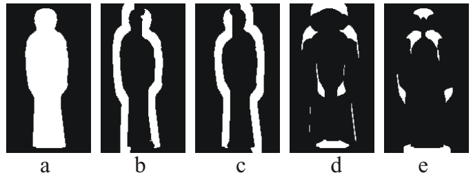
Fig. 5: a) Average Human Shape; Displacement templates: b) left, c) right, d) up, e) down
