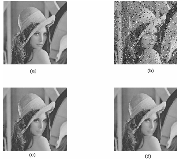
Fig.2 Lena image (a) Input image (b) Image corrupted with variance 0.1 (c)ALRWMF(d)ALRWMF-Simultaneous noise removal
