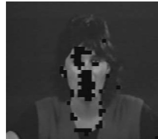
Figure 5. Reconstructed frame based on vectors found in localized codebooks, as shown in the block diagram of Fig. 2. Black areas were not encoded properly in this stage and are searched for best match in adjacent codebooks in the second stage (Fig. 3).
