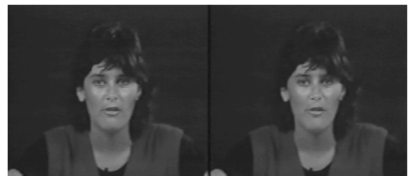
Figure 6. Original (left) and reconstructed (right) frame from the sequence Miss America, using a global codebook with 4x4x4 blocks. The compression here is 62:1.
