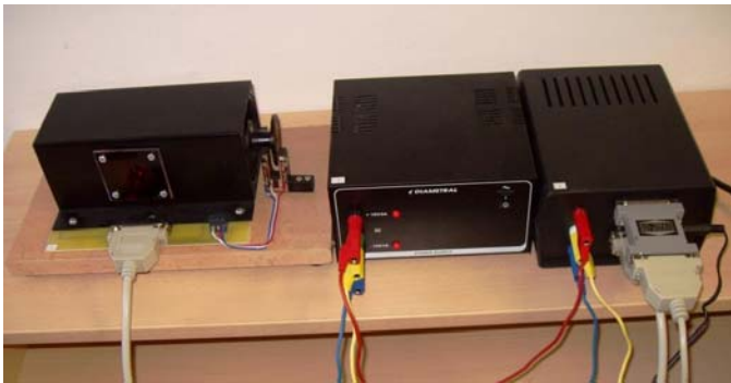
Fig. 5 Plant of HAA (from left - physical model, power supply unit, electronic module with measurement unit CTRL v3) connected to PC
