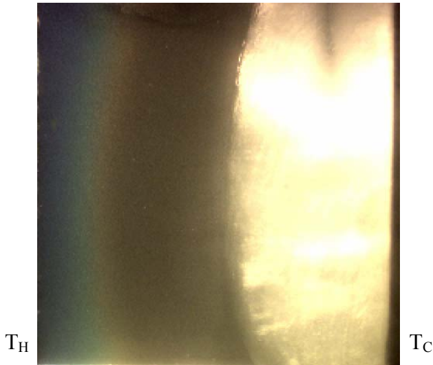
Fig.4 Steady-state free convection of 1% NaCl solution. T_H=5^{\circ}\text{C} , T_C=-5^{\circ}\text{C} . Image of the TLC's
