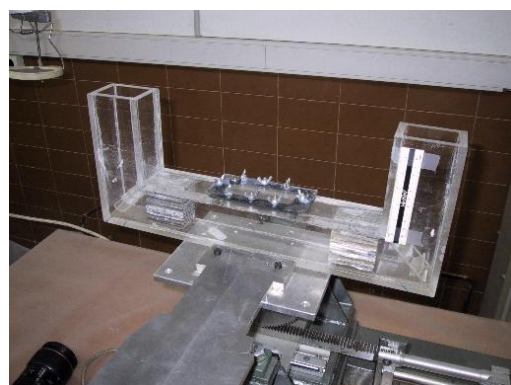
Fig.1 Water tank and the oscillation mechanism
