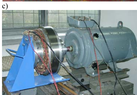
Fig. 6. View of constructional elements of the machine model constructed according to the slot cutting conception, where: a – machine stator in form of three coaxial reactive cylinders with cut teeth and a part of the associated winding. b – machine rotor in form of four coaxial field magnets, ensuring multiplied stator magnetization c – assembled machine on a test stand.
