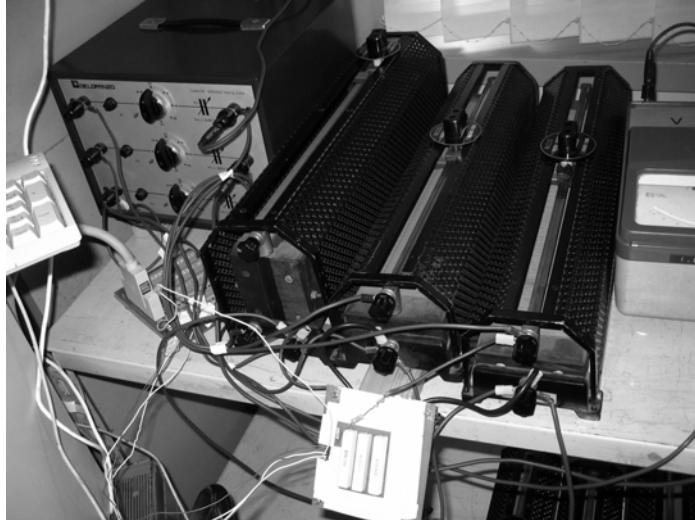
Fig. 7: The three-phase load
