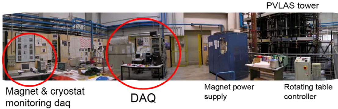
Fig. 2: panoramic view of the experimental area (november 2004). On the right the PVLAS tower is partly visible (the upper optics with the main photodiode is higher up, outside the visible area). The power supply feeds the magnet with a current greater 2000A, to reach fields as high as 6T. The DAQ hardware is assembled together, near the center of the picture.
