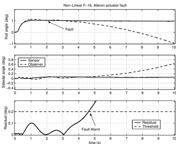
Fig. 7. Non-linear F-16 Aileron sensor fault.
