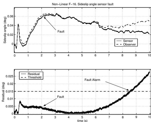
Fig. 6. Non-linear F-16 sideslip sensor fault.
