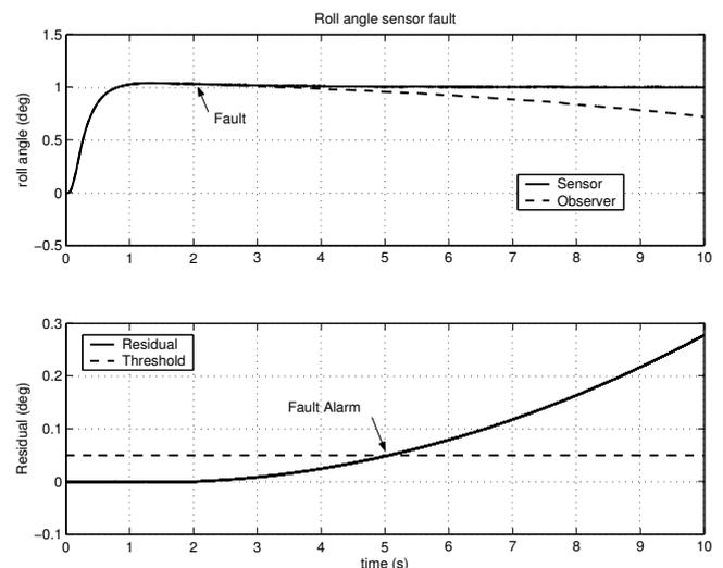
Fig. 2. Roll angle sensor fault.
