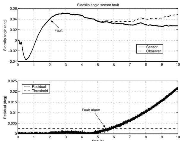
Fig. 3. Sideslip angle sensor fault.
