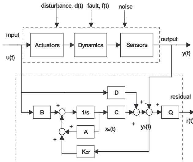
Fig. 1. Robust residual generator block diagram.
