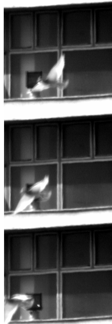
Fig. 8. A bird flying through the beam (the transceiver is located on the 7 th floor; captured from a distance of 750m).
