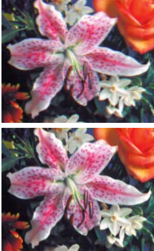
Fig.14: CCD reconstruction for the image 'Lily' with size 186x230. Top: bilinear interpolation; Bottom: the new approach.
