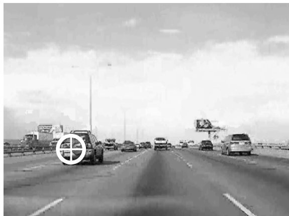
Fig. 3 Collision Avoidance Detector. Cars near a moving vehicle are located.
