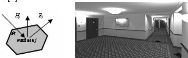
Fig. 2. Principle and design of the radiosity method
