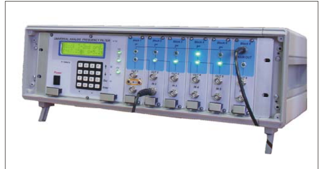
Fig.12 Resulting realization of digitally controlled analog filter unit
