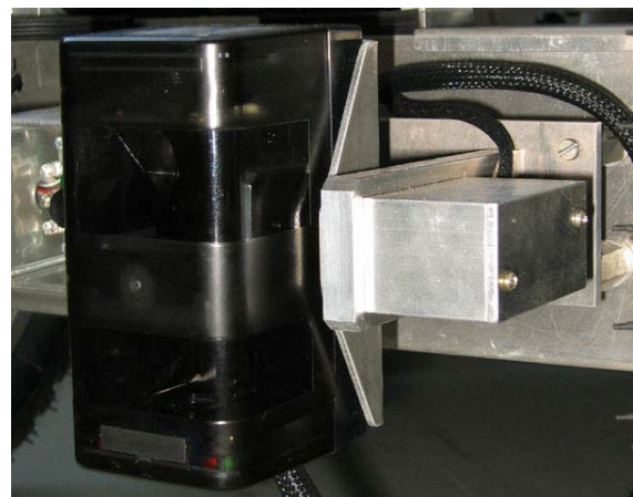
Fig. 8. Detail of 3D proximity scanner mounted on Orpheus robot
