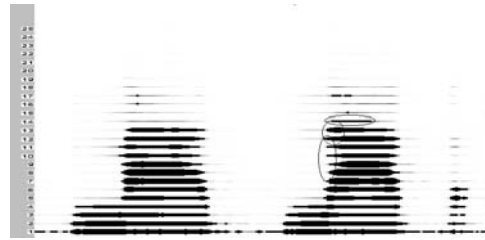
Figure 3: Filter-bank features of signal of Figure 1. Thickness of the line is an indicator of energy of feature.
