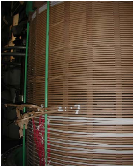
Fig.3 400kV transformer high voltage winding
