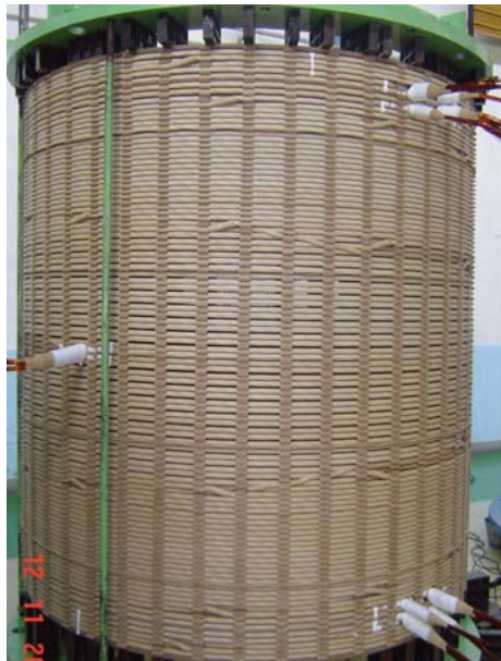
Fig 4 500kV transformer high voltage winding
