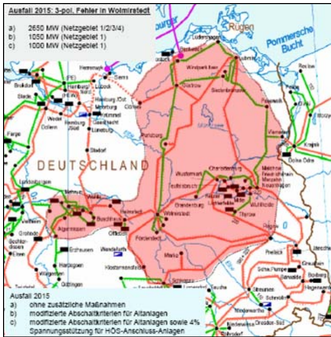
Figure 7: Part of German net in case of 3 phase short circuit in Wolmirstedt [5]
