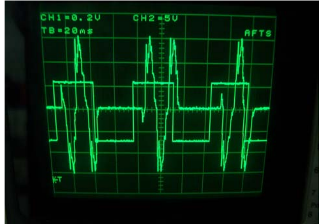
Fig.7 When SCC is used, line current waveforms of the capacitors and control signal in 16Hz control signal.
