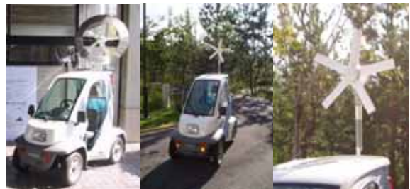
Fig.7 Appearance of EV Mounted Windmill
