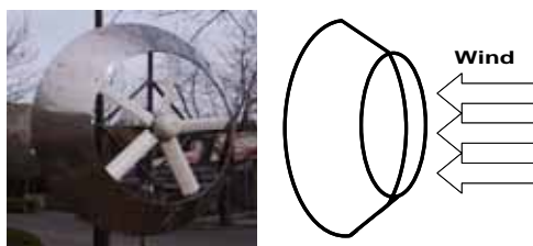
Fig.1. Wind Collection Equipment (Expanded type)
