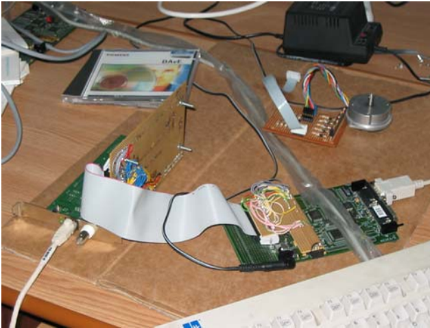
Fig. 4 – The Ethernet enabled controller
