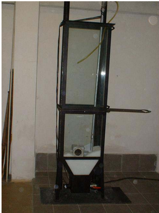
Fig.6. An actual model of a silo with details of the indicator and filling in progress. Source: Laboratory for Bulk Solids, Assoc. Prof. Jiri Zegzulka, Ph.D.
