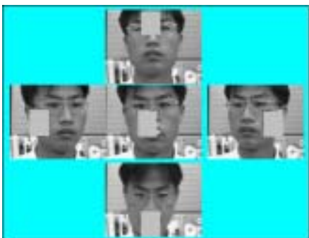
Figure 10. Results of gaze tracking using template matching
