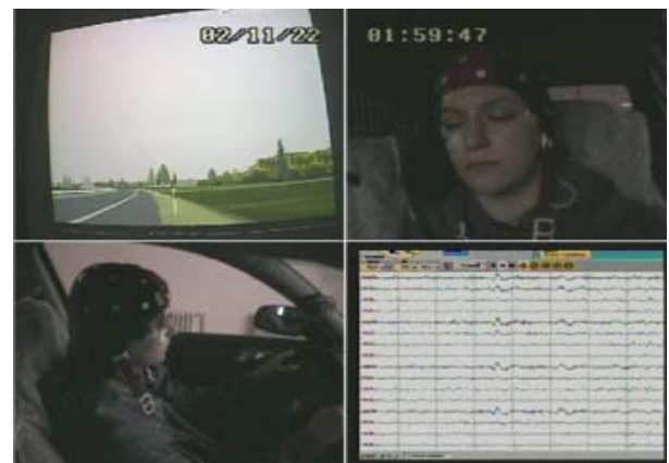
Figure 6: Video record with EEG, the proband just goes out of the road due to a micro-sleep
