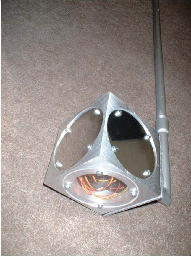
Fig.10. The 3Dimensional detector assembling for bulk solid observations. Source: [9]
