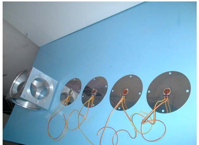
Fig.9. The load-bearing base of the cube with four deformation faces furnished with deformation detectors (tensometric sensors) connected to the full bridge. Source: [9]
