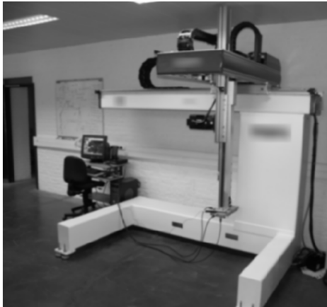
Fig. 7 – Overview of an industrial robot (stroke [mm]: X-1000 Y-400 Z-800, maximum speed: 120m/min, maximum acceleration: 4m.s -2 ).
