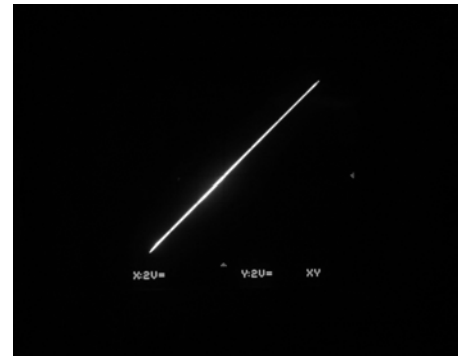
Fig.19. v_{C2} -coupling for C_2=5.30nF , C_1=8.00nF and R_C=1.3K\Omega ( v_{C22} vs. v_{C21} ). Chaotic synchronization.
