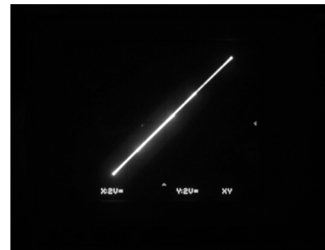
Fig.22. v_{C2} -coupling for C_2=5.30nF , C_1=8.40nF and R_C=1.5K\Omega ( v_{C22} vs. v_{C21} ). Chaotic synchronization.
