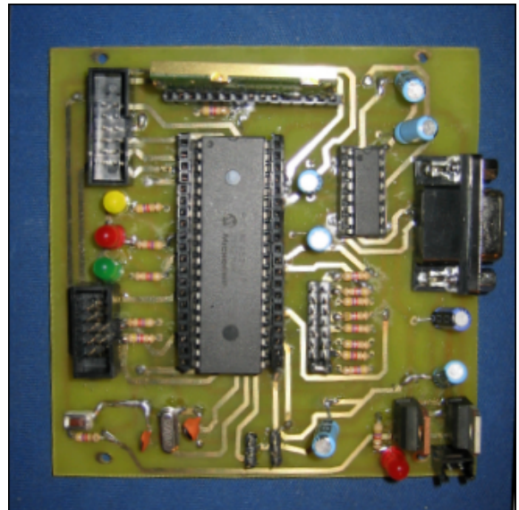
Figure 3: Control logic board.
