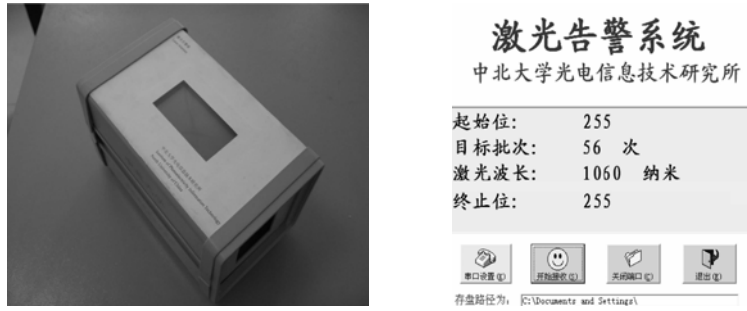
Fig.3 The prototype of laser warning receiver and display results
