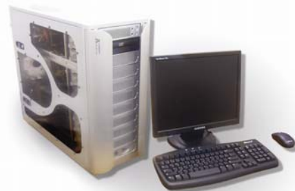
Fig. 5. Desktop supercomputer. Here we see our desktop supercomputer platform, with a Pentium 4 microprocessor, NVIDIA GeForce 7800 GTX GPU, and Celerity™ FPGA-based accelerator, shown in perspective to a standard monitor, keyboard, and mouse.
