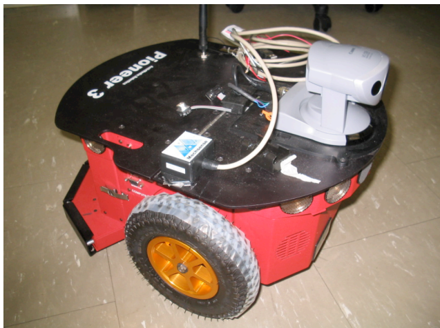
Fig. 3: Pioneer P3DX with mounted accelerometer
