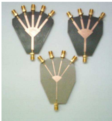
Fig.4 A Photograph of 4-way and 5-way microstrip sector power dividers.
