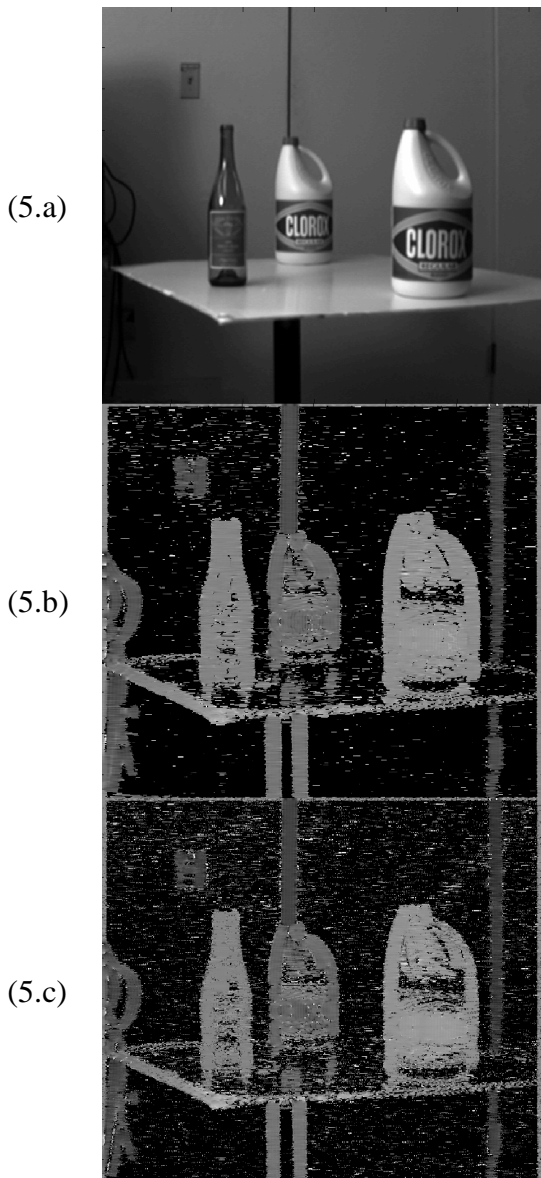
Fig. 5. Stereo processing qualitative results. a) Original image. b) Software results. c) Hardware results. Depth is encoded in grey levels.
