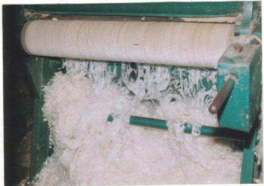
FIGURE 7 : CLOSEUP OF DOUBLE ROLLER GINNING MACHINE MOUNTED WITH RUBBERIZED COTTON FABRIC ROLLERS
