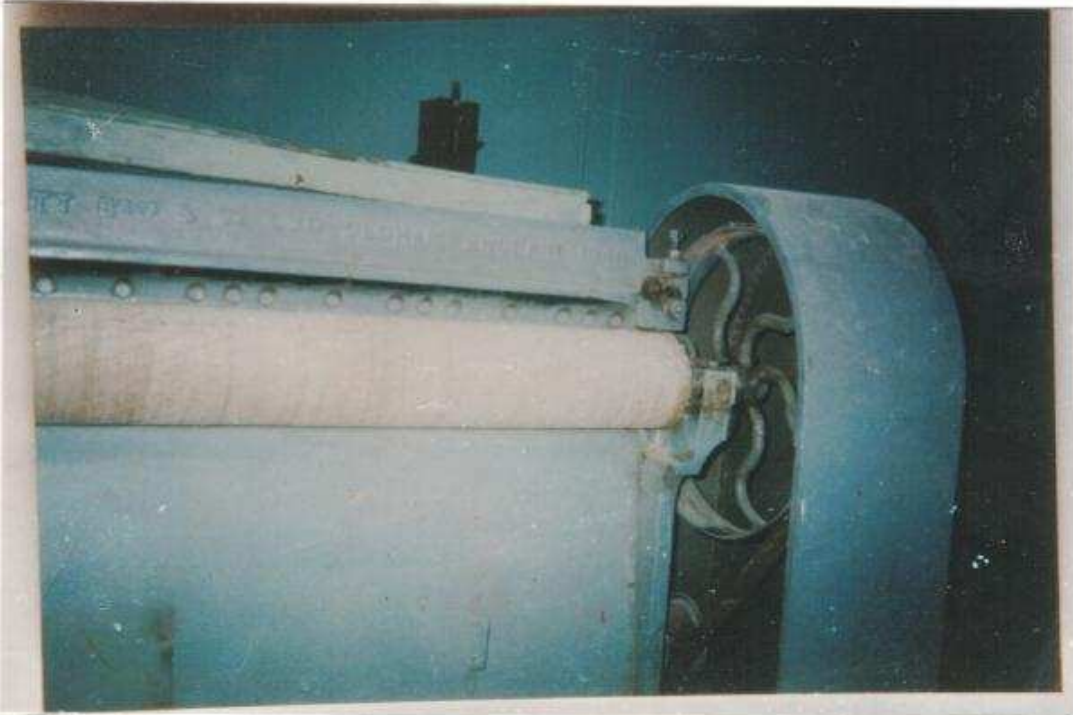
FIGURE 2 : CLOSEUP OF COTTON ROLLER GINNING MACHINE
