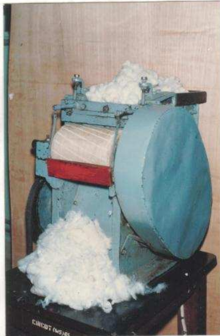
FIGURE 5 : CLOSE UP OF GIN ROLLER EXPERIMENTATION DEVICE (GRED)
