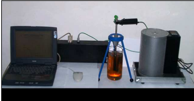
Fig. 1. Portable quenching media tester type OGJ-01, at a laboratory testing stand
