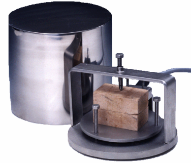
Figure2. The sample arrangement and the metallic cylinder used for guarding
