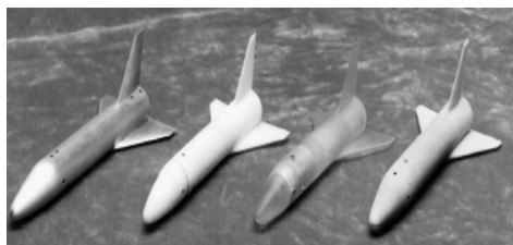
Fig. 2- Wing-body models tested (left to right), aluminum, FDM-ABS, SLA, and SLS
