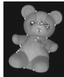
Fig.4. Interest points extracted by the Harris detector.
