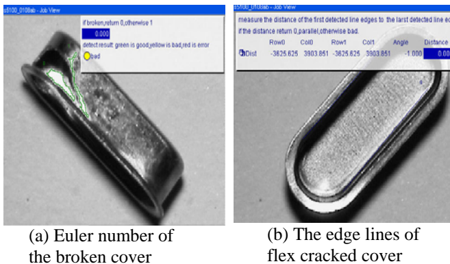
Fig.5 Detected results of the two classic types of defects
