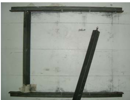
Figure 11. The device placed on the shaking table for avoiding block's rotation around the vertical z -axis and sliding.
