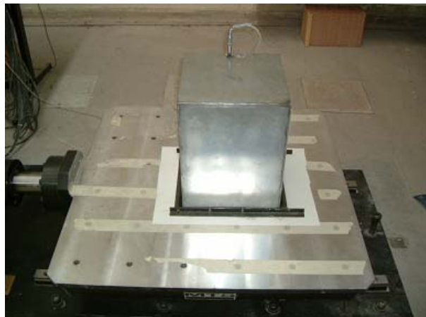
Figure 13. The 30×30×40 aluminum parallelepiped placed on the shaking table.
