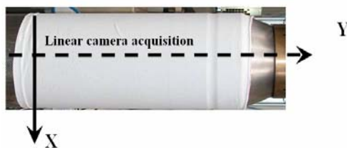
Fig.1: knitted fabric wrapped on the horizontal rotating cylinder - Provide a classification and detection error less than 10%. The detection error is evaluated with equation (1):
