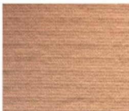
Fig.5: an example of a knitted fabric affected by a diffuse weft thread defect.
