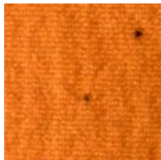
Fig.3 (left): an example of a knitted fabric affected by dark area defects.
