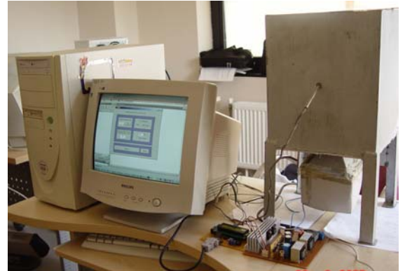
Fig. 2 the experimental temperature control system using MatLab based GUI.
