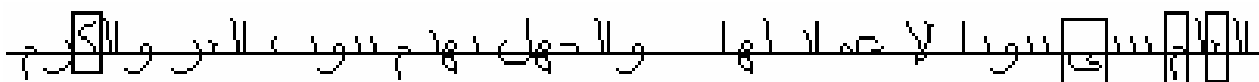
Fig. 3: The line of text after thinning and dots removal showing the main line and the bounding rectangle of some characters
