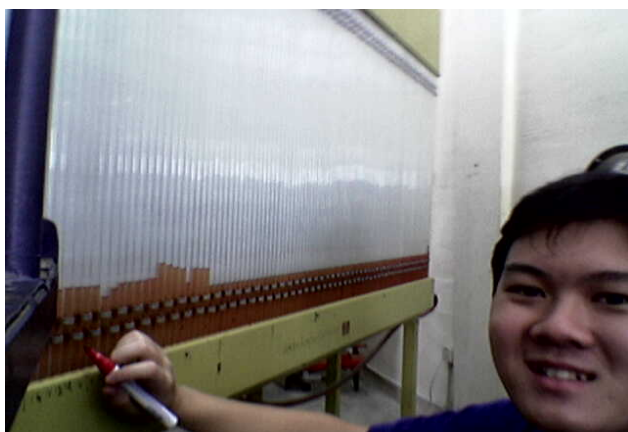
Figure 9. Taking reading from the manometer
