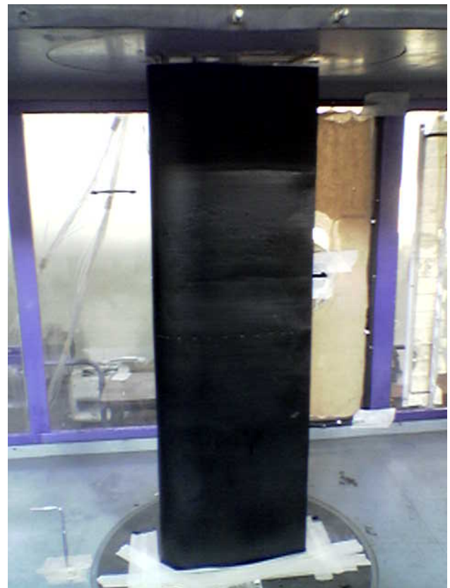
Figure 8. The test model is fixed in the test chamber of wind tunnel (with 32 flush orifices).
