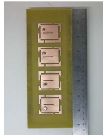
Fig.6 Proposed rectangular microstrip array antenna with asymmetric T-shaped slit loads.
