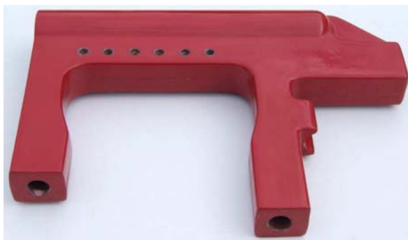
Fig. 10 Main part to sustain the chair executed from sandwich composites materials.
