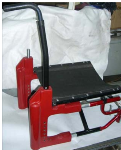
Fig. 9 Structure for the wheel chair from polymeric composites materials
