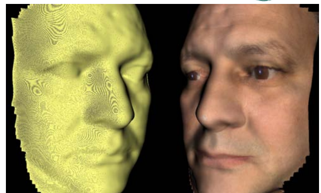
Fig 6: Top: estimating the point cloud from equations 3-5 and building a triangulated mesh with texture mapping from the stripe colour scheme. Bottom: texturing with a colour bitmap.
