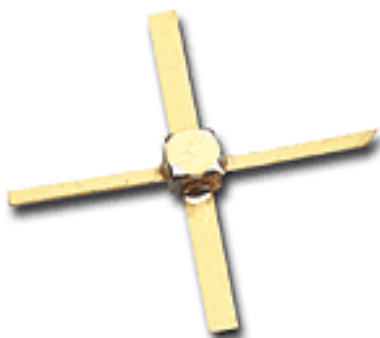
Figure 1.b. Ceramic Packaged MMIC amplifier model MSA-0670 from Agilent Technologies.
